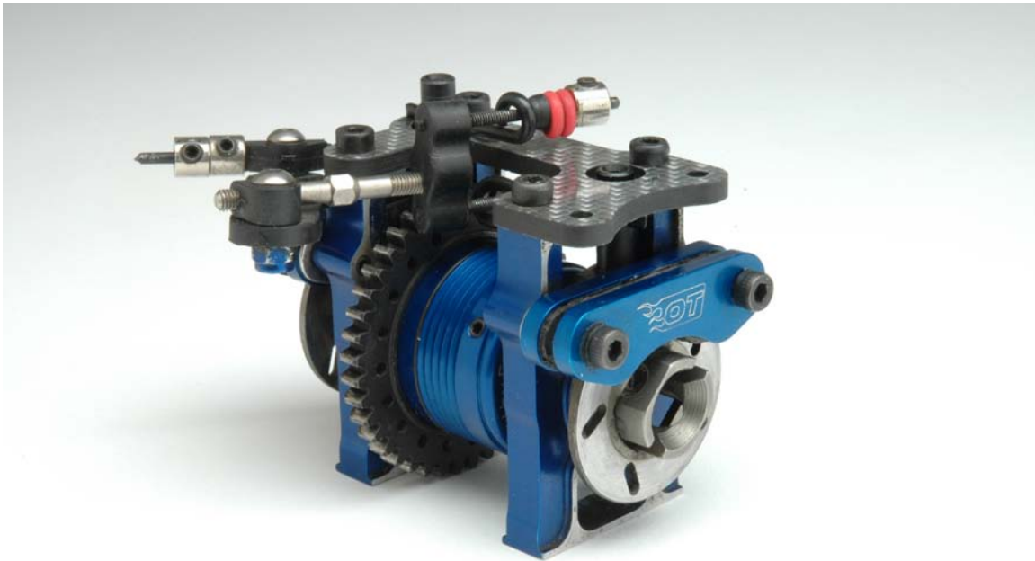
Center Diff Mount, Aluminum Diff Housing, and Brake Calipers
